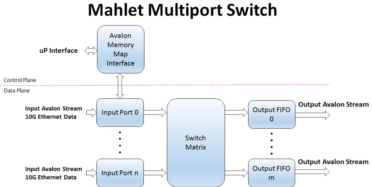
Figure 1: Mahlet MPS Block Diagram
